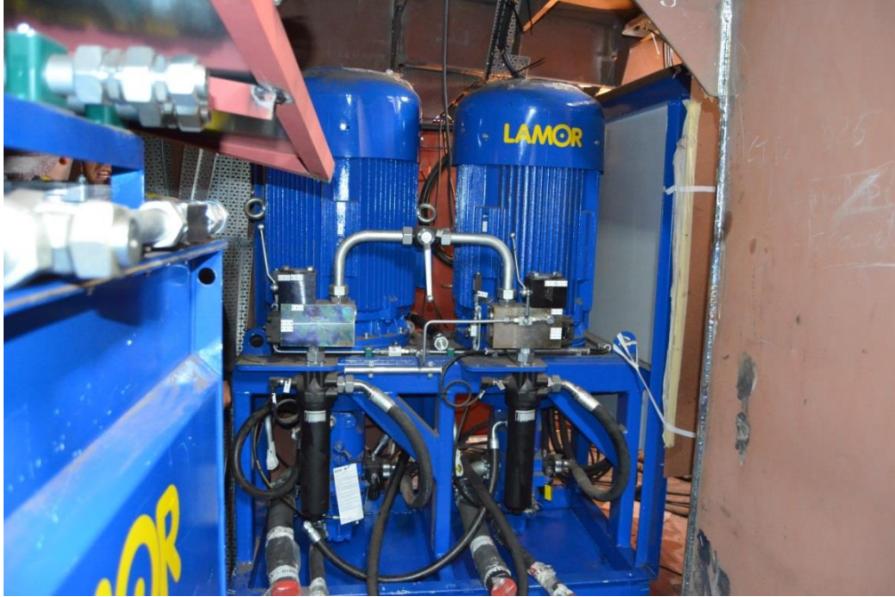
Fig.11 Power pack frame and electric motors 2 x 90kW
